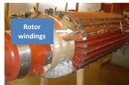
Figure 8 - Generator rotor
