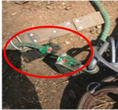
Figure 2. Pictures of safety belt configuration with cut braided safety line
