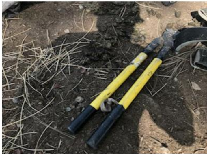
Figure 3. Lopper style cutters
