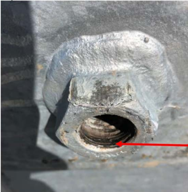
Stripped bolt used to hold hydraulic jack in place
