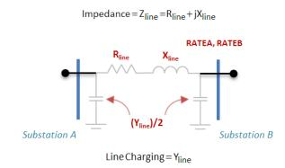
Figure 14 - Transmission line model uses impedance values, but converts these to a "Y-bus" matrix using line admittances.
