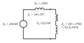
Figure 22 - A simple circuit with actual voltage, current, and impedance values.
