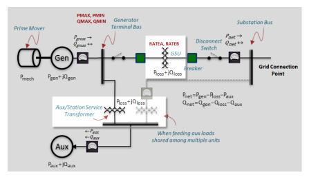
Figure 15 - Generator step-up and auxiliary transformers
