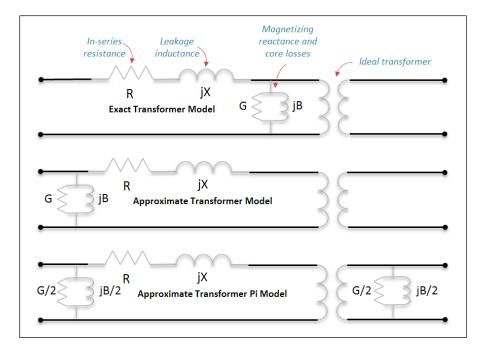
Figure 20 - Transformer equivalent circuit models
