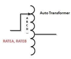
Figure 16 - The autotransformer has a common winding that it tapped to provide the desired secondary voltage. Taps are typically on the high side, but can be on the low side.
