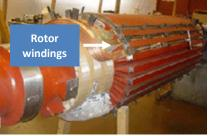
Figure 8 - Generator rotor
