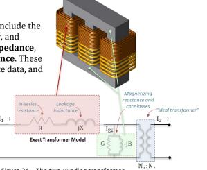
outside the magnetic core path. The magnetizing conductance, Figure 24 – The two-winding transformer equivalent model.
