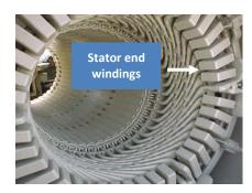
Figure 9 - Generator stator
