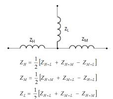
Figure 26 - Three-winding transformer modeled as a "star" or "T " or "T."
