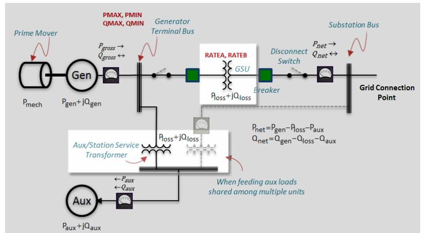
Figure 15 - Generator step-up and auxiliary transformers
