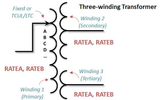
Figure 17 - Three-winding power transformer that can be used to supply loads at two different voltages.
