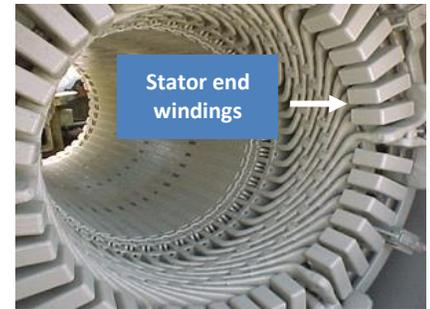
Figure 9 - Generator stator
