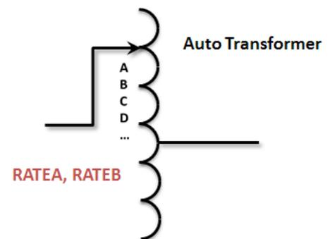
Figure 16 - The autotransformer has a common winding that it tapped to provide the desired secondary voltage. Taps are typically on the high side, but can be on the low side.
