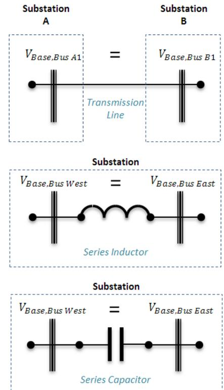
Figure 2 - The base voltage for busses connected by lines or series reactive equipment must be the same.
