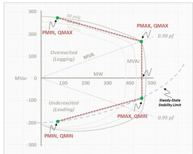
Figure 10 - Piecewise linear representation of the generator limits, PMAX, PMIN, QMAX, QMIN.
