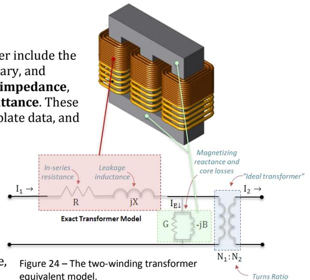
Figure 24 – The two-winding transformer equivalent model.
