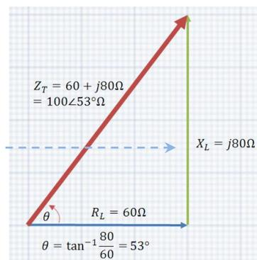
Figure 23 - Converting the circuit impedance from R+jX to vector form.
