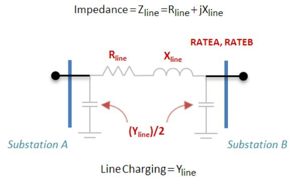
Figure 14 - Transmission line model uses impedance values, but converts these to a “Y-bus” matrix using line admittances.
