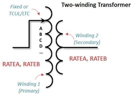
Figure 18 –Two-winding power transformer. This one allows for voltage regulation by adjusting the tap setting. Either side can be tapped, but taps are typically on the high side.
