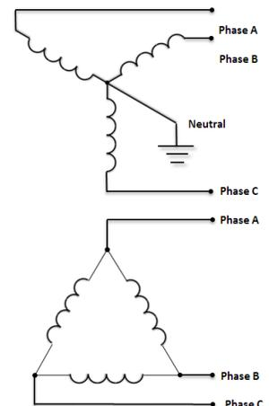
Figure 25 - It's possible to convert the "T" model into a Delta model (bottom), but the lack of an artificial center node may result in negative impedances that can be difficult for some power flow programs to solve.
