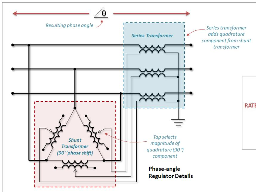
Figure 19 - The phase angle regulator comprises a shunt and series transformer to produce the desired phase angle. The internal details are shown at left, and the model representation below.
