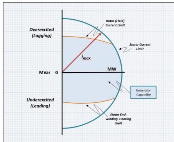
Figure 5 - The operating limits of the generator are bounded by the rotor current limits during lagging operation and stator end winding heating during leading operation. The result is a “D” curve, which is the shaded part of the graph.
