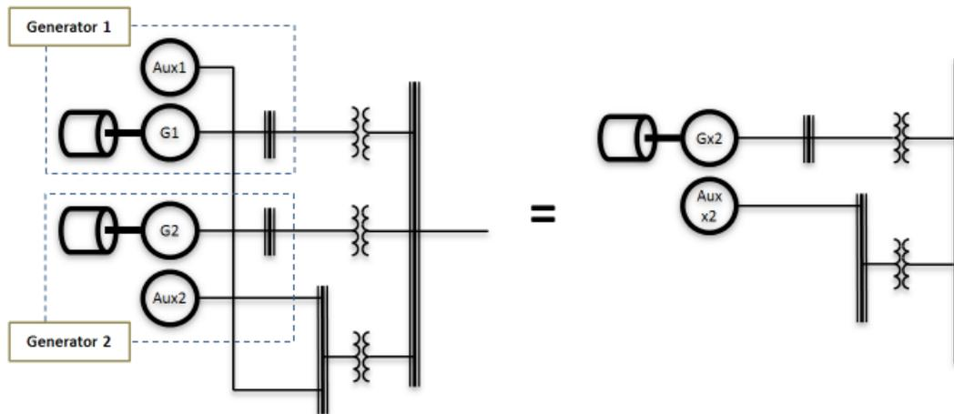
Figure 13 - Generators at the same plant may be combined into a single equivalent generator if the individual units have the same characteristics.
