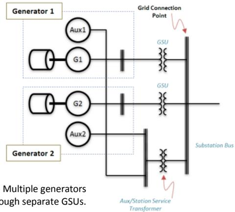
Figure 12 - Multiple generators connected through separate GSUs.
