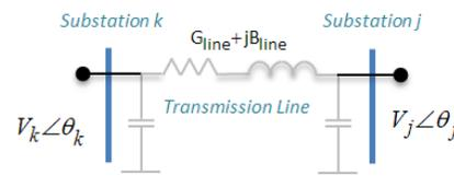
Figure 1 - Transmission line model using Y-bus representation
