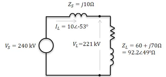
Figure 22 - A simple circuit with actual voltage, current, and impedance values.
