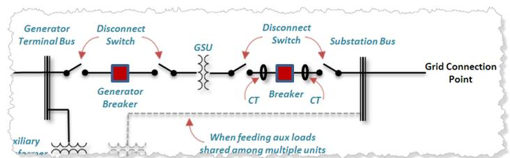
Figure 4 - Switchgear includes disconnect switches and current and potential transformers.
