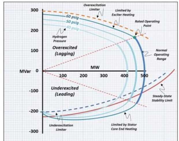
Figure 7 - D-curve with other limits shown.
