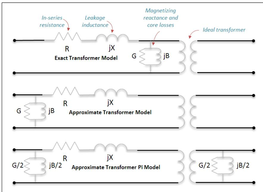
Figure 20 - Transformer equivalent circuit models
