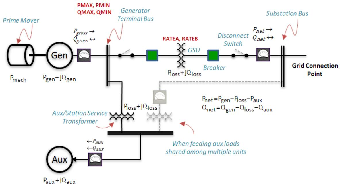
Figure 3 - Generating plant model details
