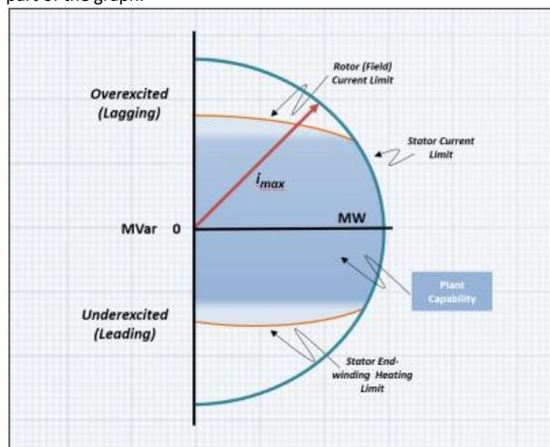
Figure 6 - The plant rating includes the limits of the up- and down-stream equipment, such as the prime mover and down-stream auxiliary equipment or step-up transformer.
