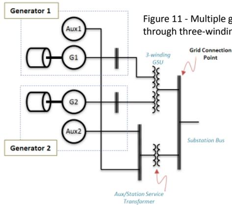
Figure 11 - Multiple generators connected through three-winding GSU.
