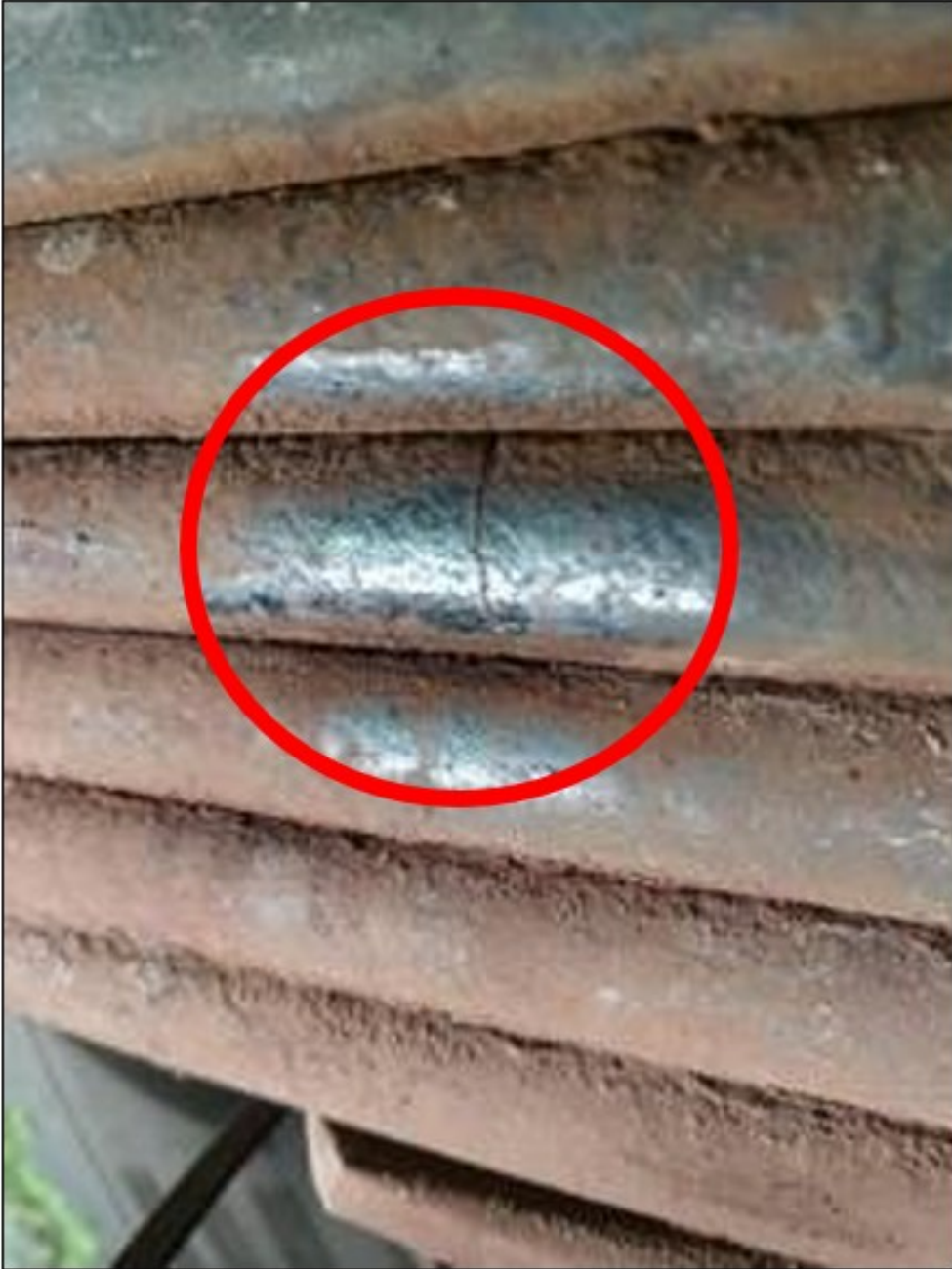
Figure 1 - Broken Leaf Spring
