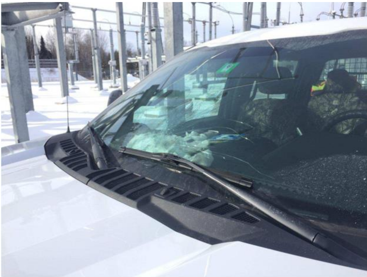
View of the burned area of the truck dashboard. Snow was used to extinguish the fire.
