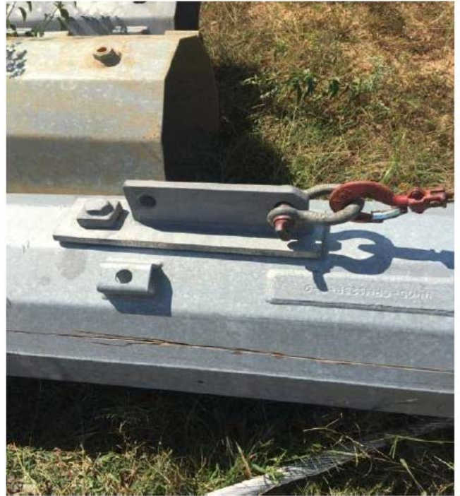
New Plate - load transferred to surface of nut
