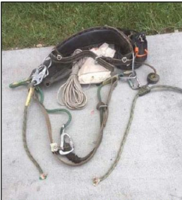
Figure 1: Apprentice Lineman No. 1's Fall Restriction Equipment (FRE). Note the rope safety that broke as a result of being drilled through.
