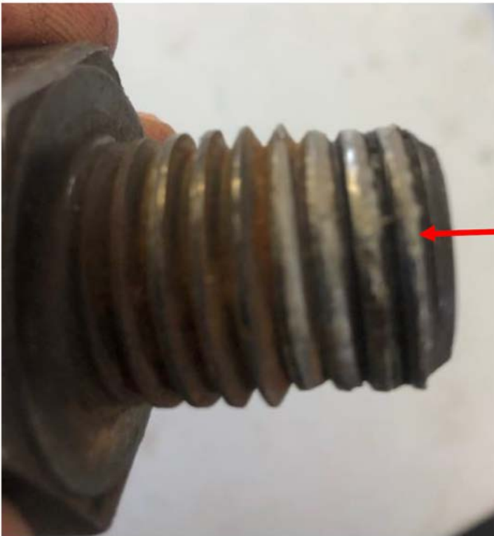
Stripped bolt used to hold hydraulic jack in place
