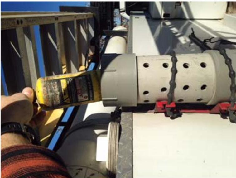
Brass propane cap required to be used on all disposable tanks not in use:
