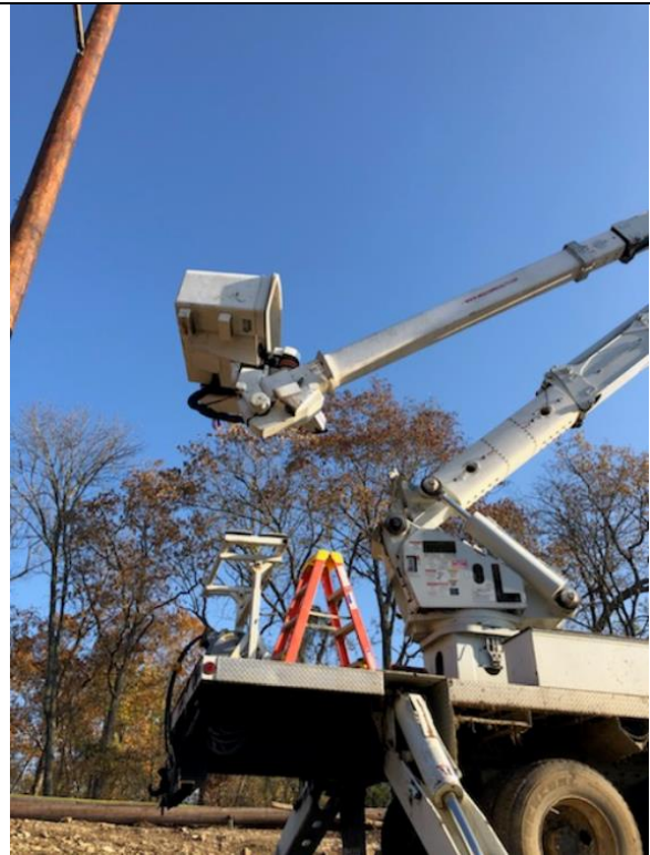
Side view as left because it would not return to stowed position.
