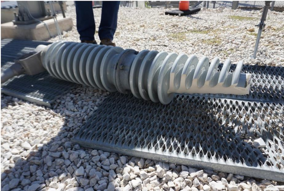
Figure 2. Portion of Failed Insulator and Buss that Fell to Ground
