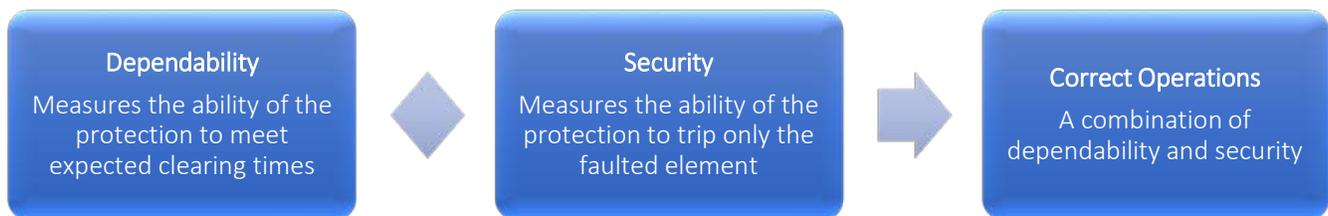
A small number of misoperations are failures to trip or slow trips, which are reflected in the dependability metric. The majority of misoperations are unnecessary trips, which drives the security metric lower. The separate metrics provided by the NATF initiative help us understand the nature of misoperations and, in some cases, see how different protection system design philosophies affect the balance between dependability and security.
